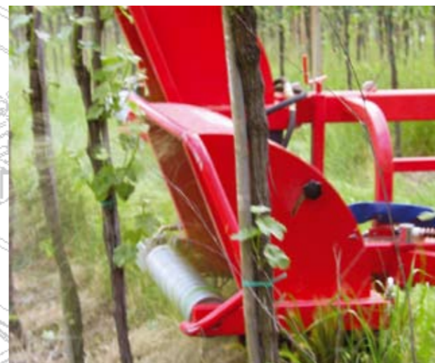
Spollonatrice con rotore in nylon - Tipping with nylon rotor
